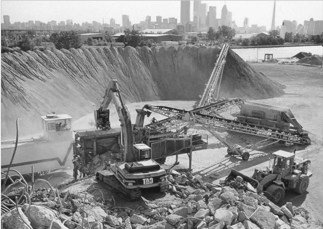
An aggregates recycling operation in Toronto. Such operations can help conserve resources and reduce waste.
